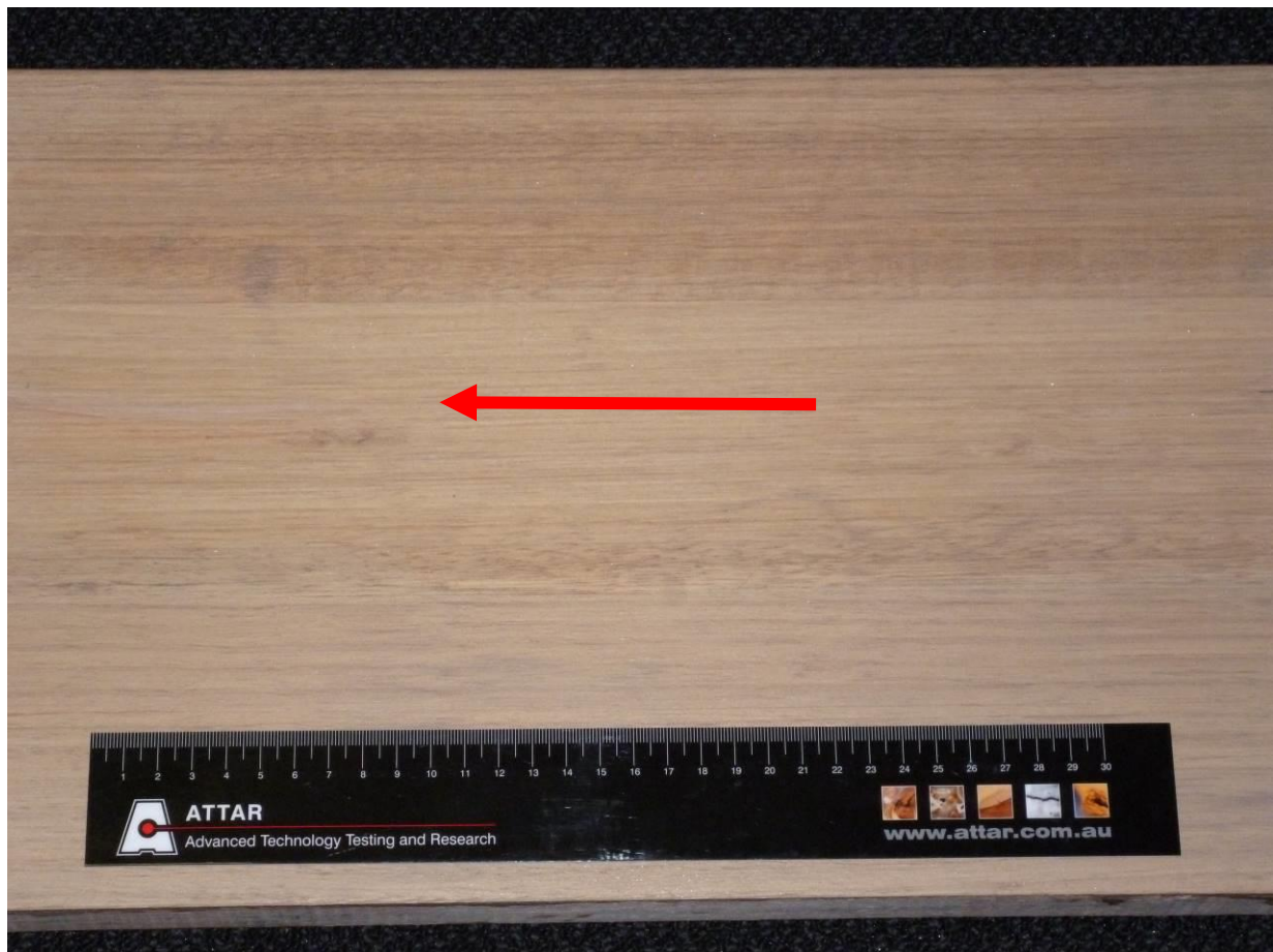
Figure 1: Microfloor Skid Resist 50 applied to Mountain Ash hardwood in accordance with manufacturer's instructions. Arrow indicates direction of test.
